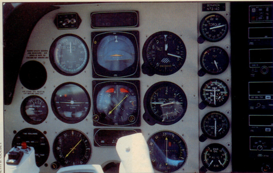
The new Bonanza panel appears to have been designed to accommodate turbine gauges. A fuel totalizer (left of the ADF) enables accurate measure of fuel consumption.
