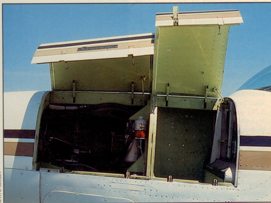
Forward cowling door allows access to the turbine engine and engine accessories. Rear door opens on a baggage locker that can hold up to 150 pounds of luggage.
